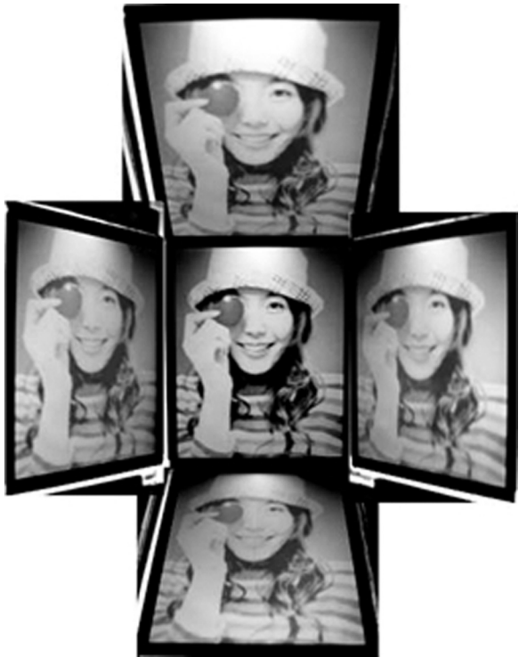
FIGURE 5 PNLCD panel images with crossed polarizer taken at various viewing angle.
